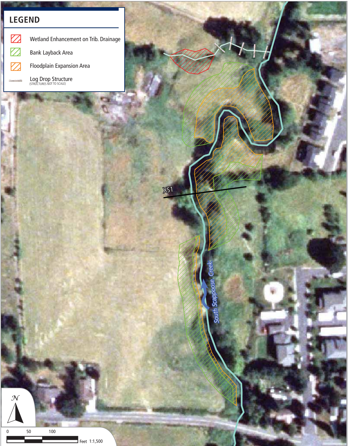
FIGURE 2: Plan view of conceptual channel restoration design options on property owned by the City of Scappoose adjacent to Veterans Park.
