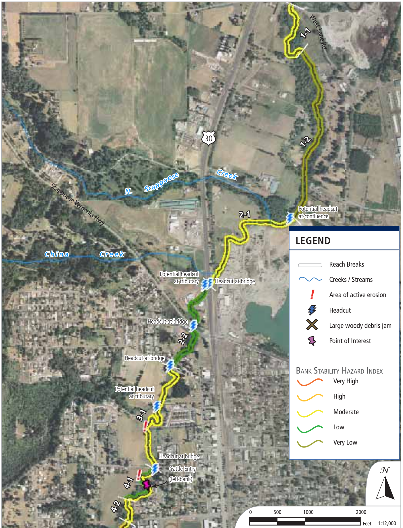
FIGURE 16: A bank and channel stability survey was conducted on South Scappoose Creek through the project area. The selected study approach, based on Rosgen (1996), produced a Bank Erosion Hazard Index (BEHI) for each bank along with site specific bank and bed stability observations. 39
